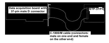
Figure 2. Connecting the STP-37/FC to the data acquisition board
